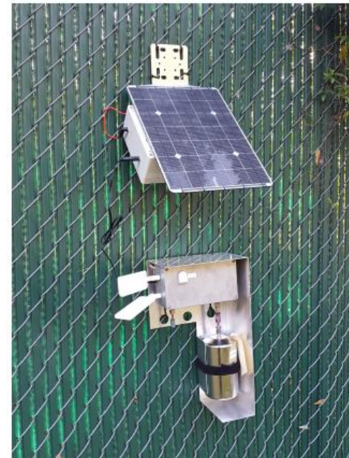
Remotely Operated Canister Sampler (ROCS) Prototype.
