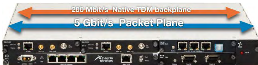
Figure 0-13: High-Speed Planes Interconnect to Deliver Highest Nodal Capacity
