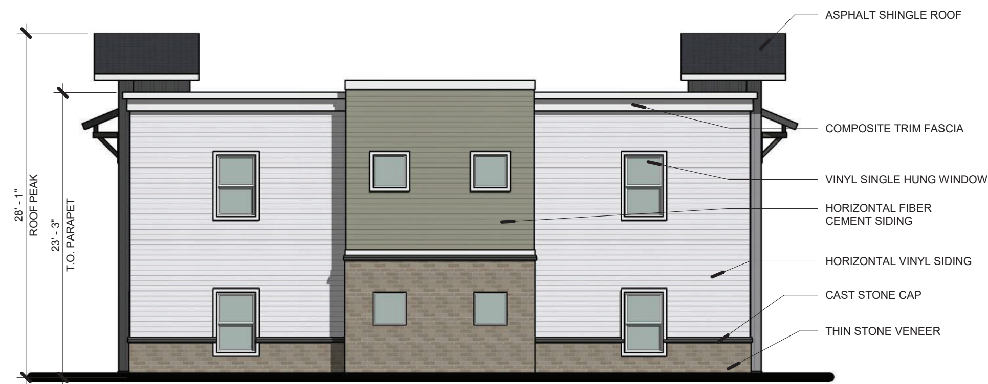
4 BLDG E - TYP. SIDE ELEVATION PR4.4 1/8" = 1'-0"
