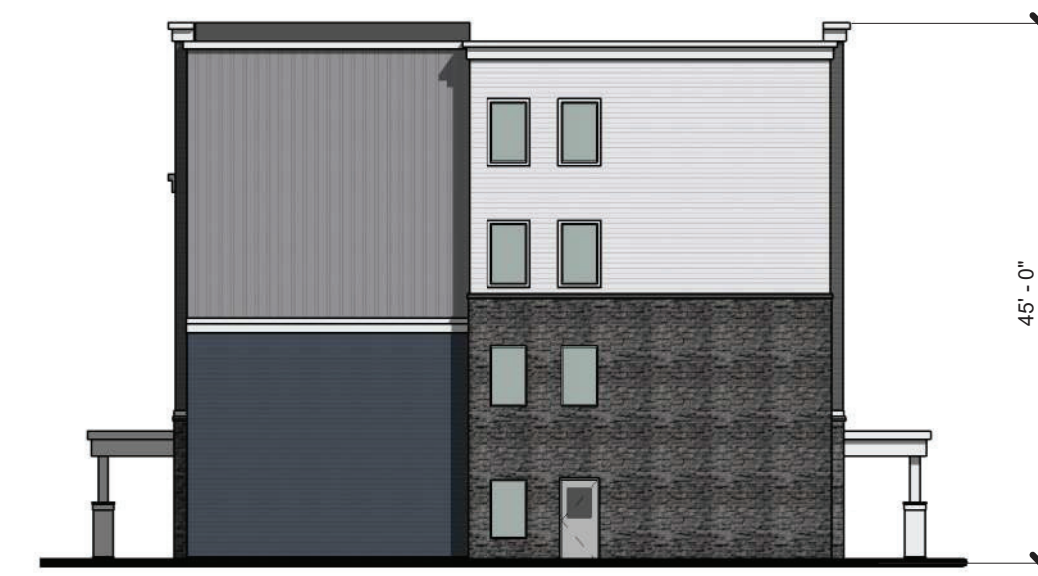
4 BUILDING A - NORTH ELEVATION PR4.1 1/16" = 1'-0"
