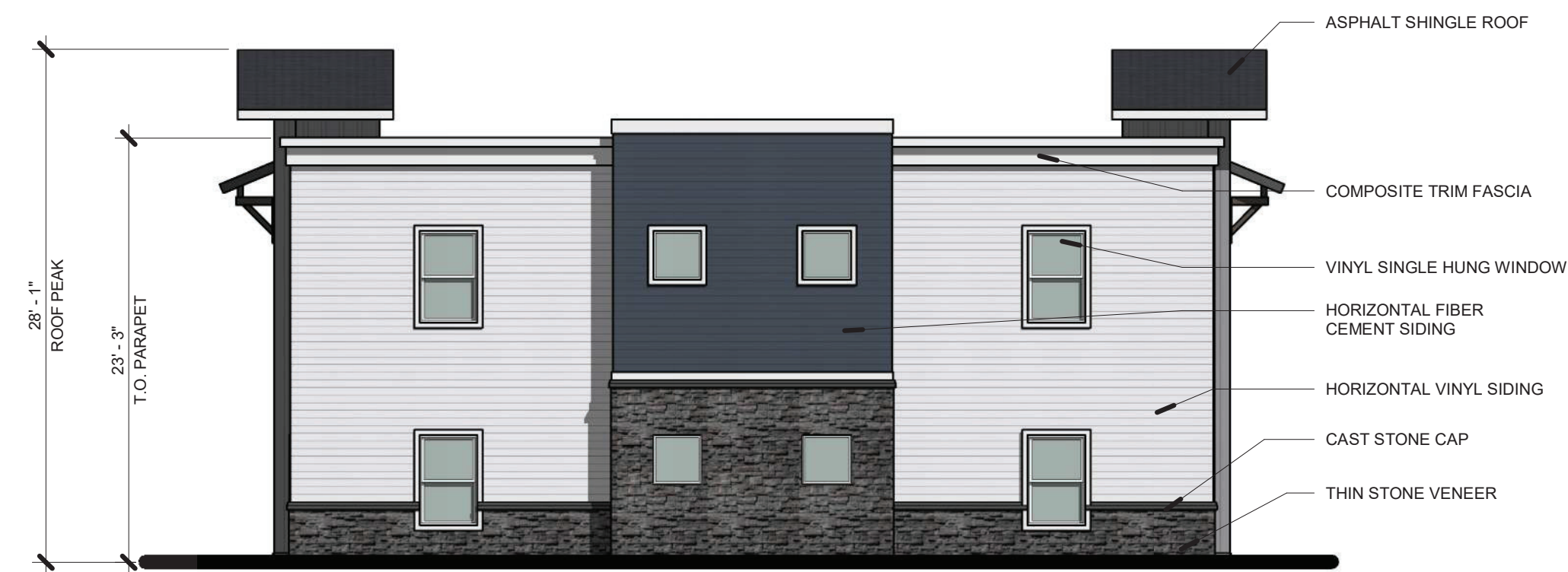
2 BLDG D - TYP. SIDE ELEVATION PR4.4 1/8" = 1'-0"
