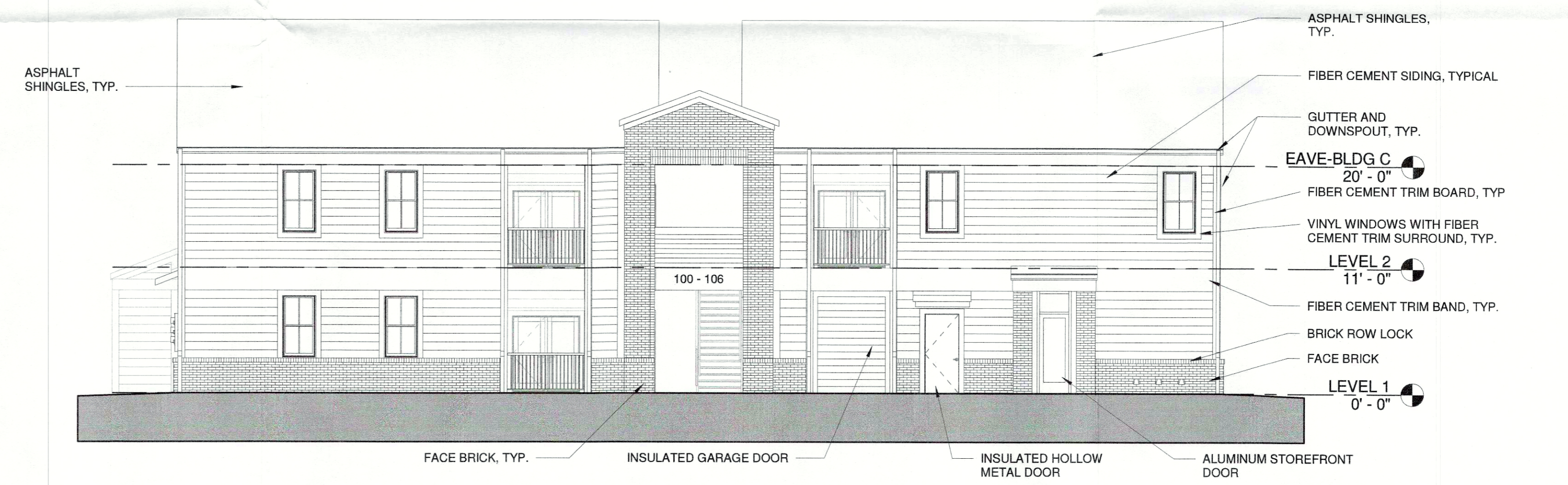
REAR ELEVATION BUILDING "C" 3 1/8" = 1'-0" A402
