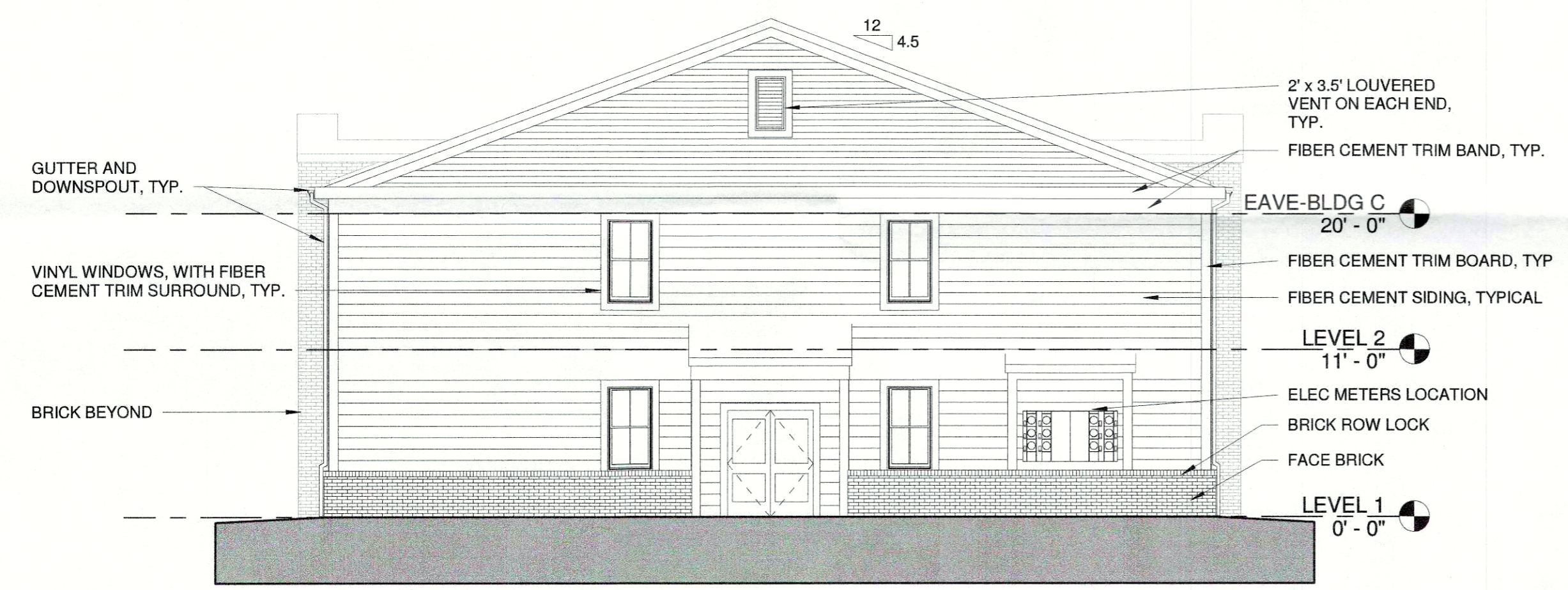
RIGHT ELEVATION BUILDING "C" 4 1/8" = 1'-0" A402
