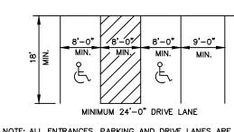
NOTE: ALL ENTRANCES, PARKING AND DRIVE LANES ARE ASPHALT, CONCRETE OR A HARD DURABLE SURFACE AS PERMITTED BY METRO PUBLIC WORKS.
