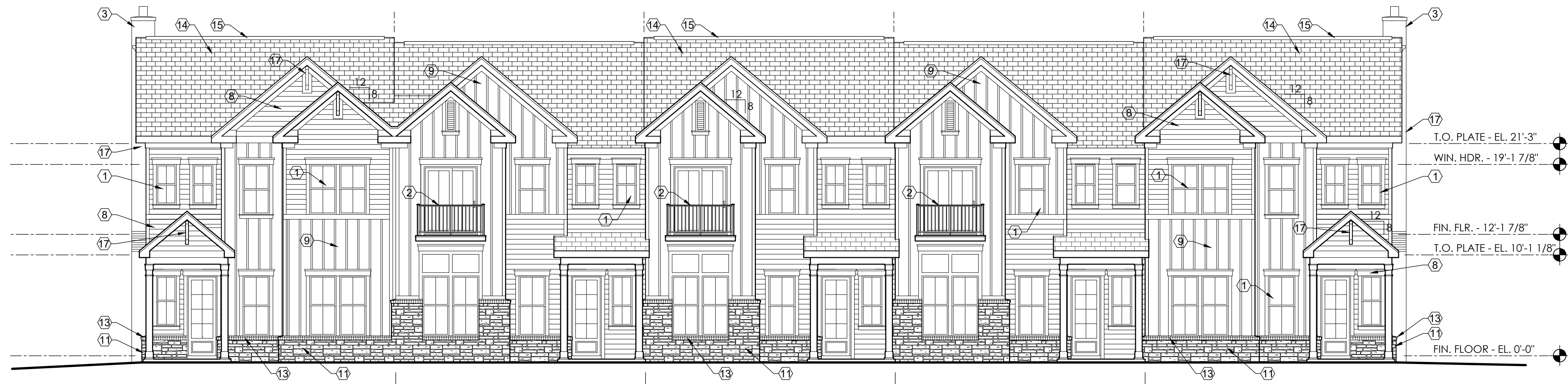
1 5-UNIT BUILDING FRONT ELEVATION SCALE: 1/8" = 1'-0" 0' 2' 4' 8' 16' 32'
