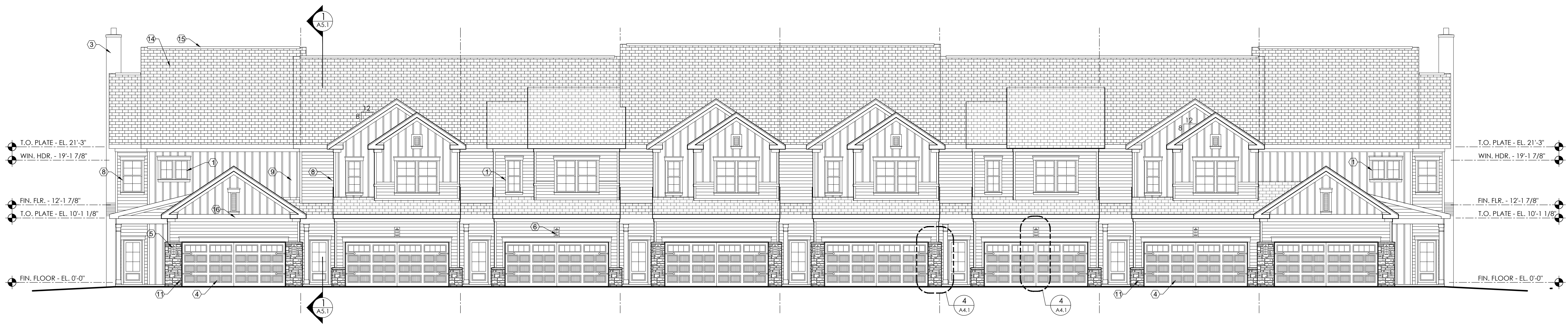
1 8-UNIT BUILDING FRONT ELEVATION SCALE: 1/8" = 1'-0" 0 2' 4' 8' 16' 32'
