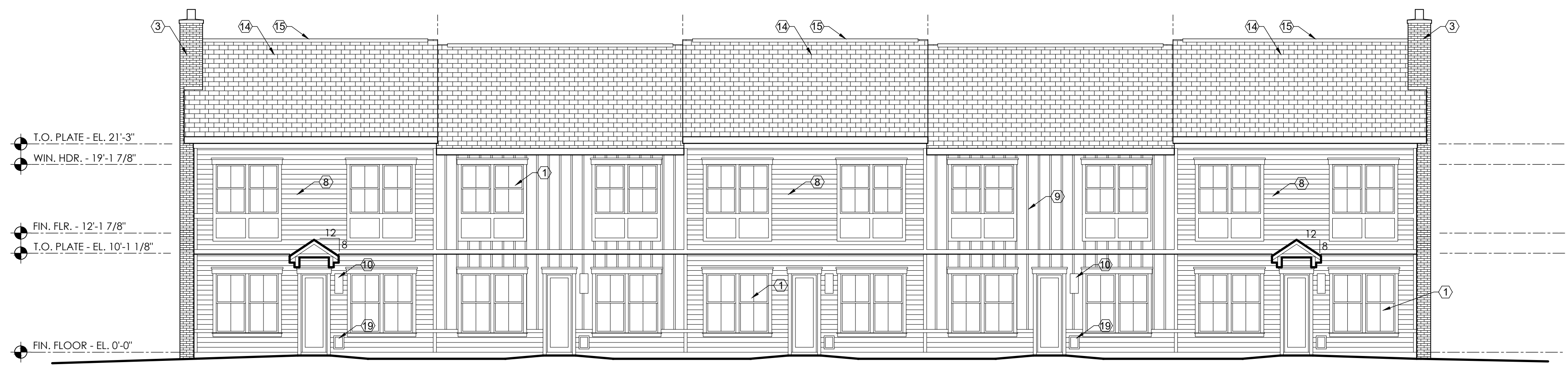
5 5-UNIT BUILDING REAR ELEVATION SCALE: 1/8" = 1'-0" 0' 2' 4' 8' 16' 32'
