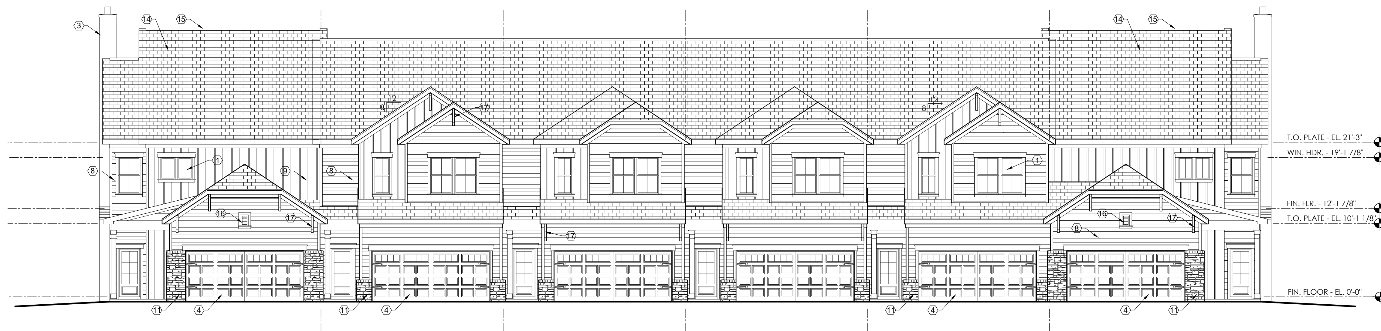
1 6-UNIT BUILDING FRONT ELEVATION SCALE: 1/8" = 1'-0" 0' 2' 4' 8' 16' 32'
