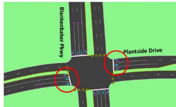
Figure 2. Recommended Lane Revisions to Plantside Drive
