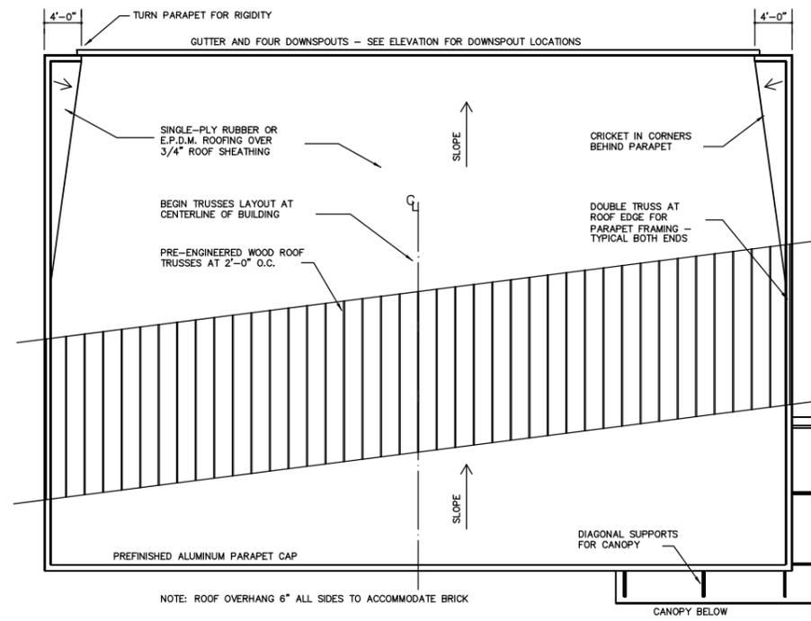
**ROOF AND ROOF FRAMING PLAN**
