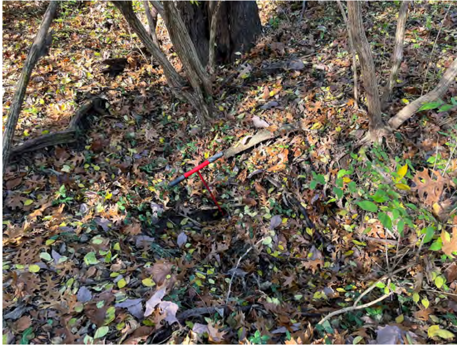
Photo 11: View of probe rod extended in partially closed throat located in F-11.
