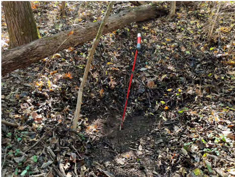
Photo 12: View of probe rod extended in partially closed throat located in F-12.
