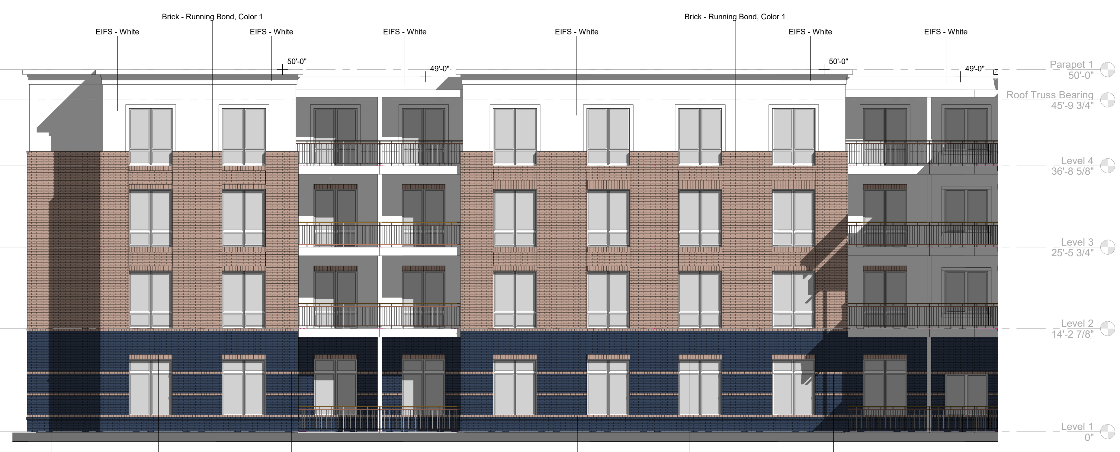
5 Courtyard 3 - West Elevation SD204 1/8" = 1'-0"
