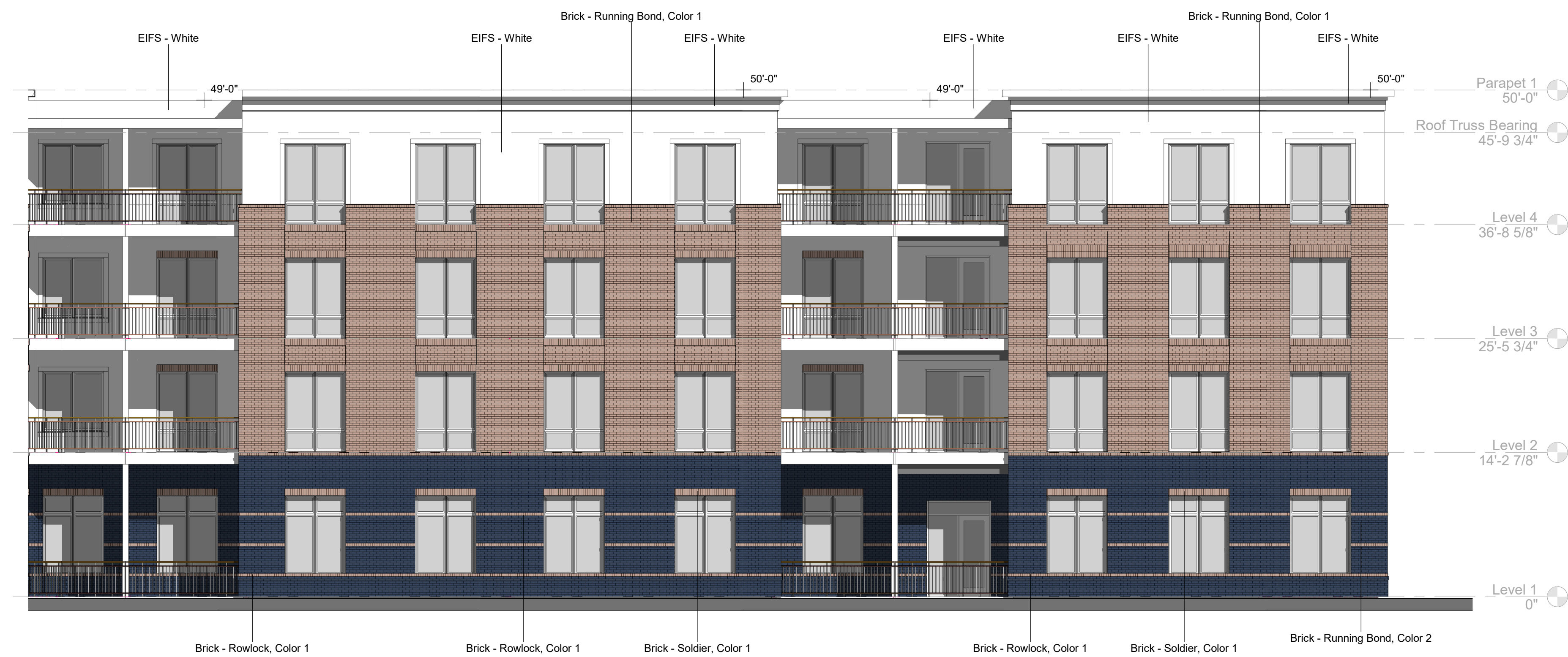
4 Courtyard 3 - East Elevation SD204 1/8" = 1'-0"
