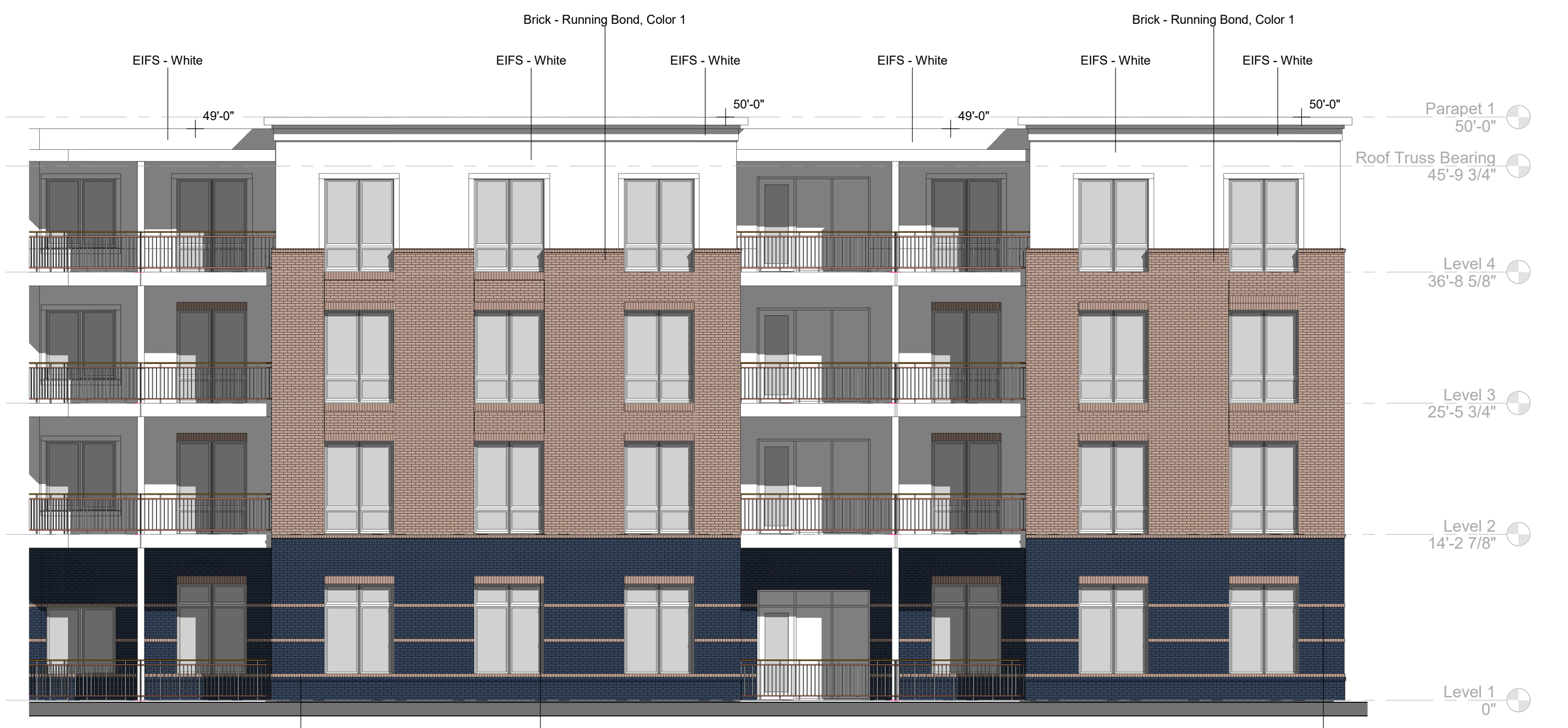
3 Courtyard 2 - East Elevation SD203 1/8" = 1'-0"
