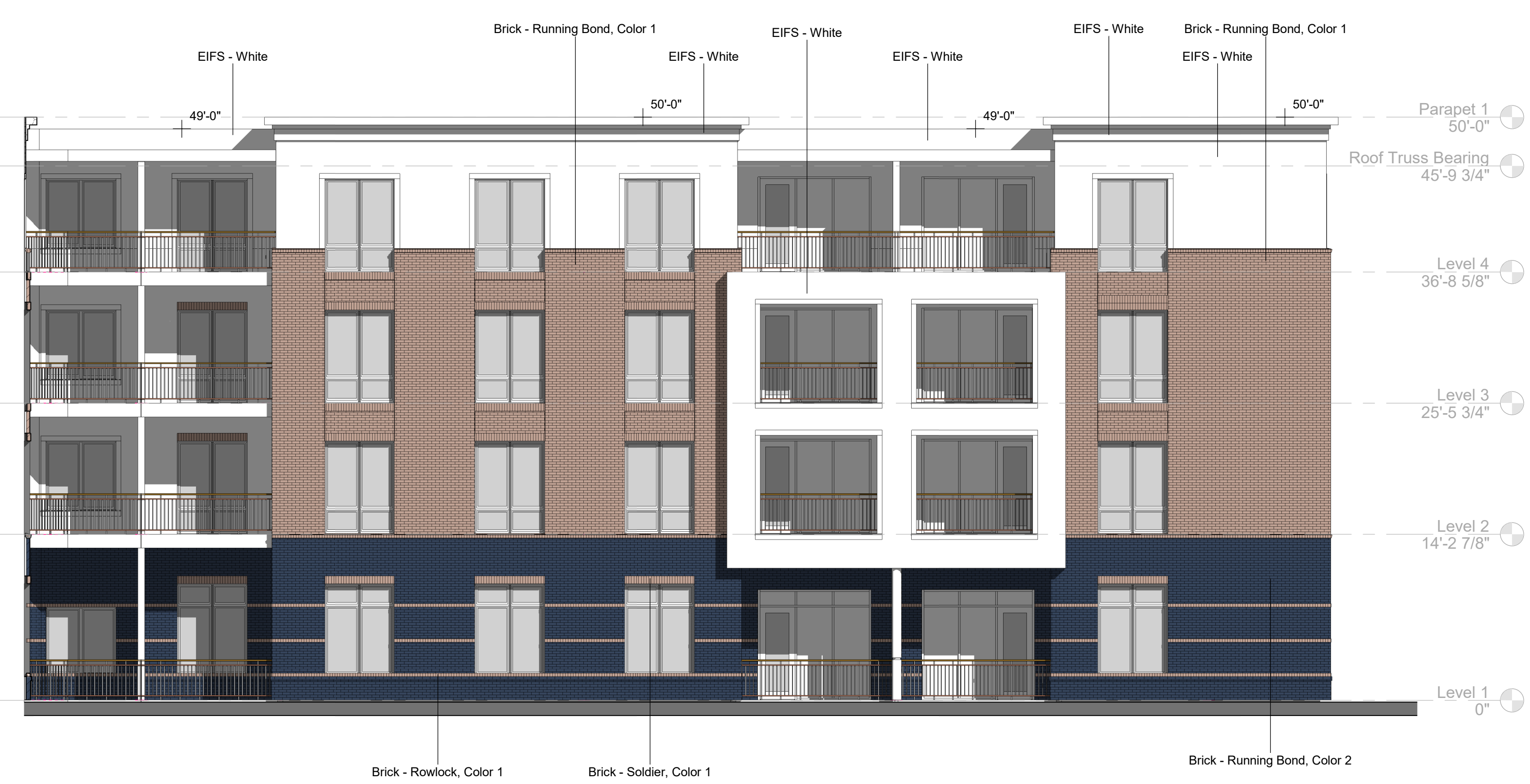
1 Courtyard 1 - East Elevation SD204 1/8" = 1'-0"
