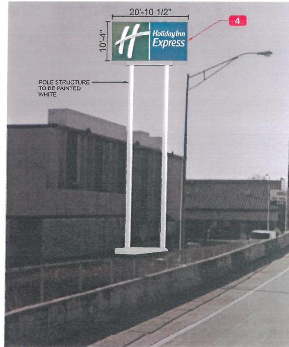
Proposed Double-Faced Internally Illuminated XHR-217 Highway Sign (217 sq. ft.)
