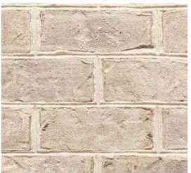
B3 : BRICK VENEER GENERAL SHALE WINDSOR WHITE OR APPROVED EQUAL BY OWNER
