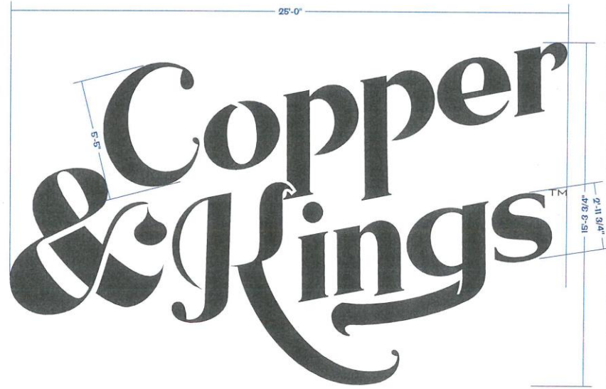
2" Aluminum Fabricated Letters Stud Mounted to Corrugated Metal Wall
