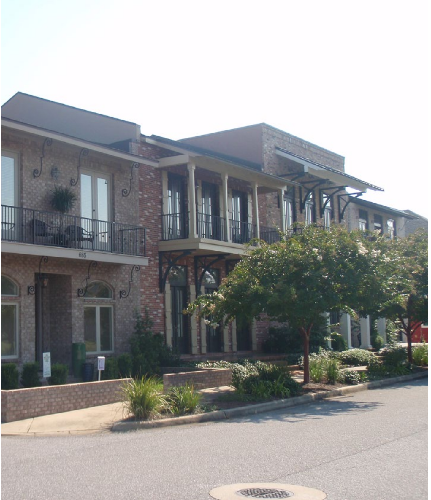
This development illustrates articulating facades through the variety of heights, roof pitches, porches, columns, and awnings.
