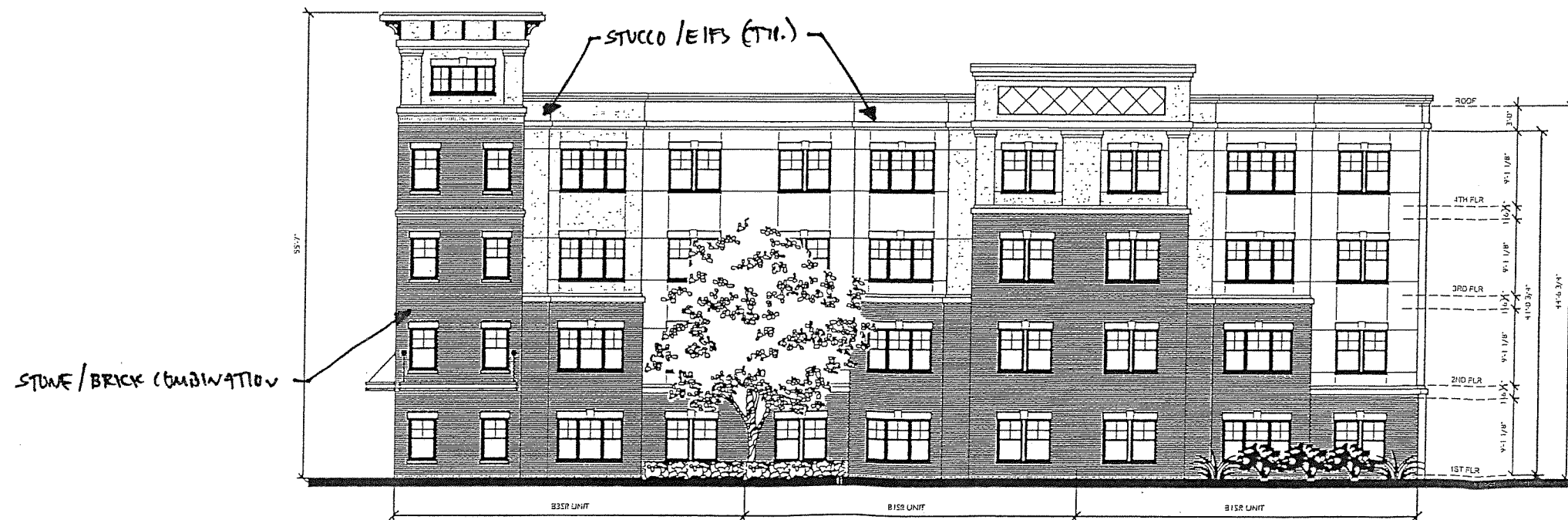
1 BLDG. TWO - WEST ELEVATION 1/8"=1'-0"
