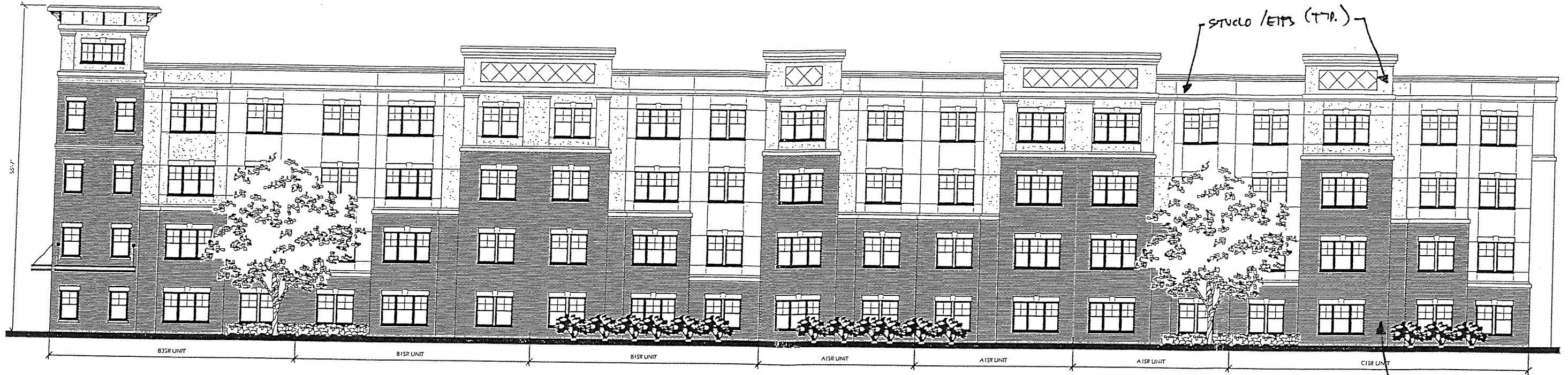
2 BLDG. THREE - NORTH ELEVATION 1/8"=1'-0"
