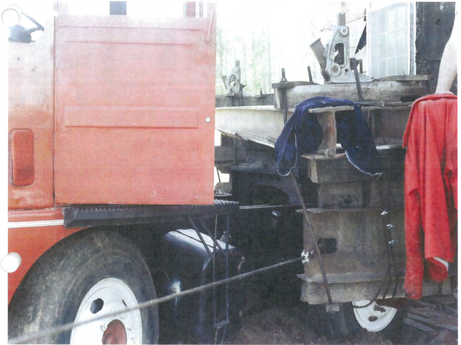
1996 - Moving truck being assisted with steel rope pulled by large wrecker.
