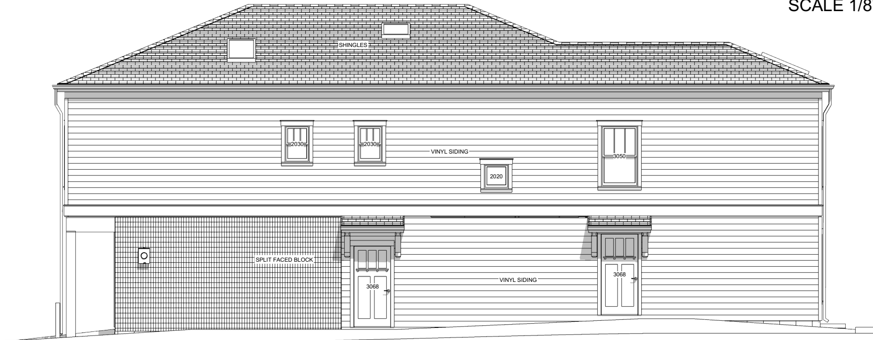
PROPOSED LEFT SIDE ELEVATION SCALE 1/8"=1'-0"
