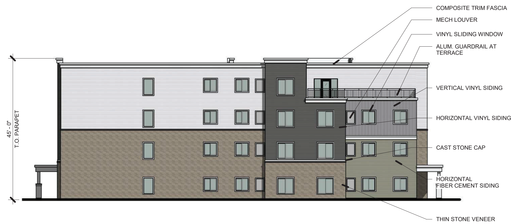
3 BUILDING C - WEST ELEVATION PR4.3 1/16" = 1'-0"
