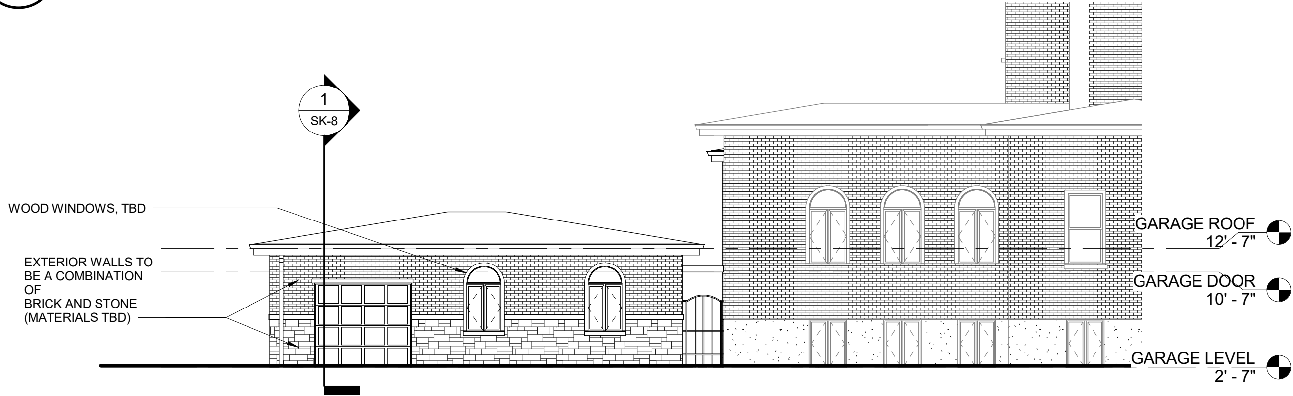
2 GARAGE ELEVATION SOUTH SK-4 SCALE: 1/8" = 1'-0"
