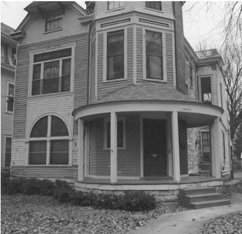
*Above, the house retains its original siding, but its porch elements have been replaced by inappropriate substitutes that do not match the visual appearance of the original.*
