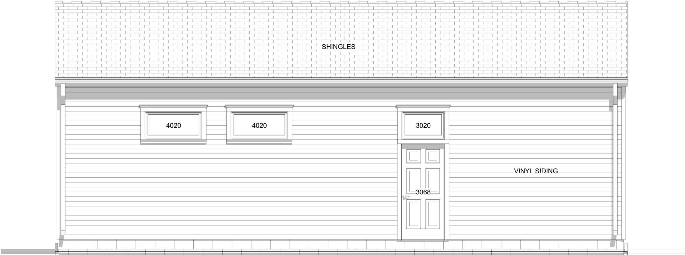
PROPOSED GARAGE REAR (YARD) ELEVATION
