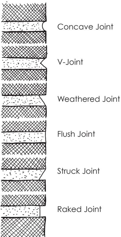
Match the existing bonding pattern, coursing, color, size, strength, and pointing mortar of the original masonry. The type of mortar joint selected can affect the visual appearance of a masonry wall and the way the wall sheds water.
