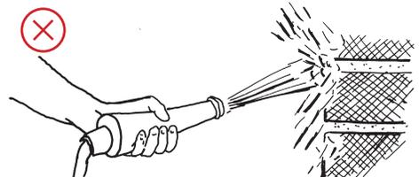
Use the gentlest means possible to clean masonry. Scrubbing with natural-bristle brushes is recommended. High-pressure water or sandblasting erodes the surface of the brick and dislodges mortar and should be avoided.
