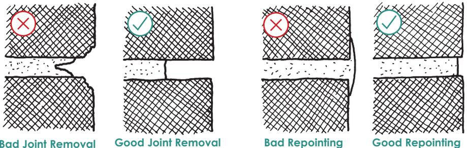
Repoint a deteriorated masonry mortar joint. Remove an unsound mortar joint by hand to a depth of two and a half times the width of the joint, or to sound mortar. Bad repointing results in brick damage from grinding tools, mortar that is too hard, and sloppy joints. Good repointing carefully removes deteriorated mortar using hand tools and replaces it with compatible mortar, slightly recessed from the edge of the brick.
