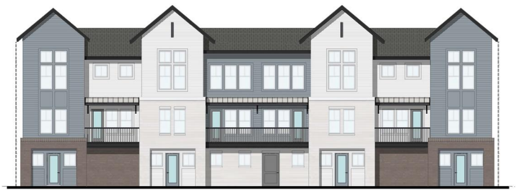
BUILDING TYPE IV - FRONT ELEVATION SCALE: 1/8" = 1'-0"
