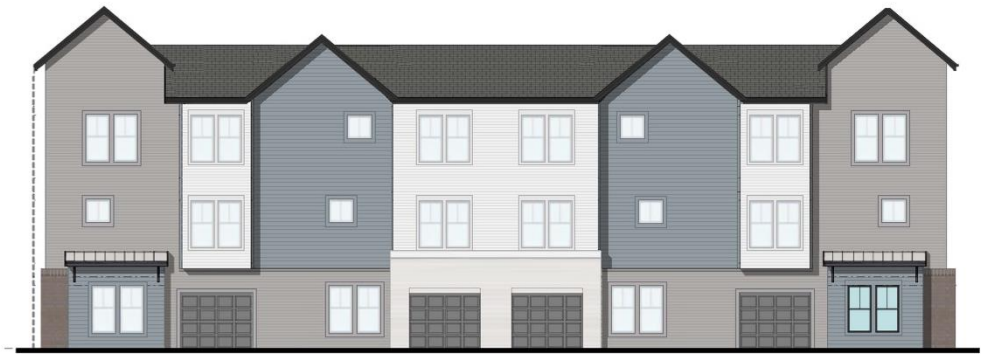
BUILDING TYPE IV - REAR ELEVATION SCALE: 1/8" = 1'-0"
