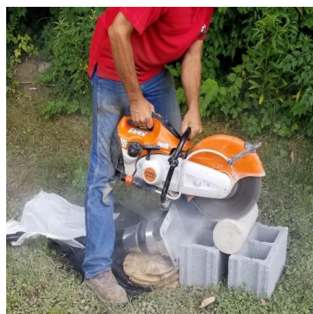
Figure 1. Image showing the dust collection method and apparatus.
