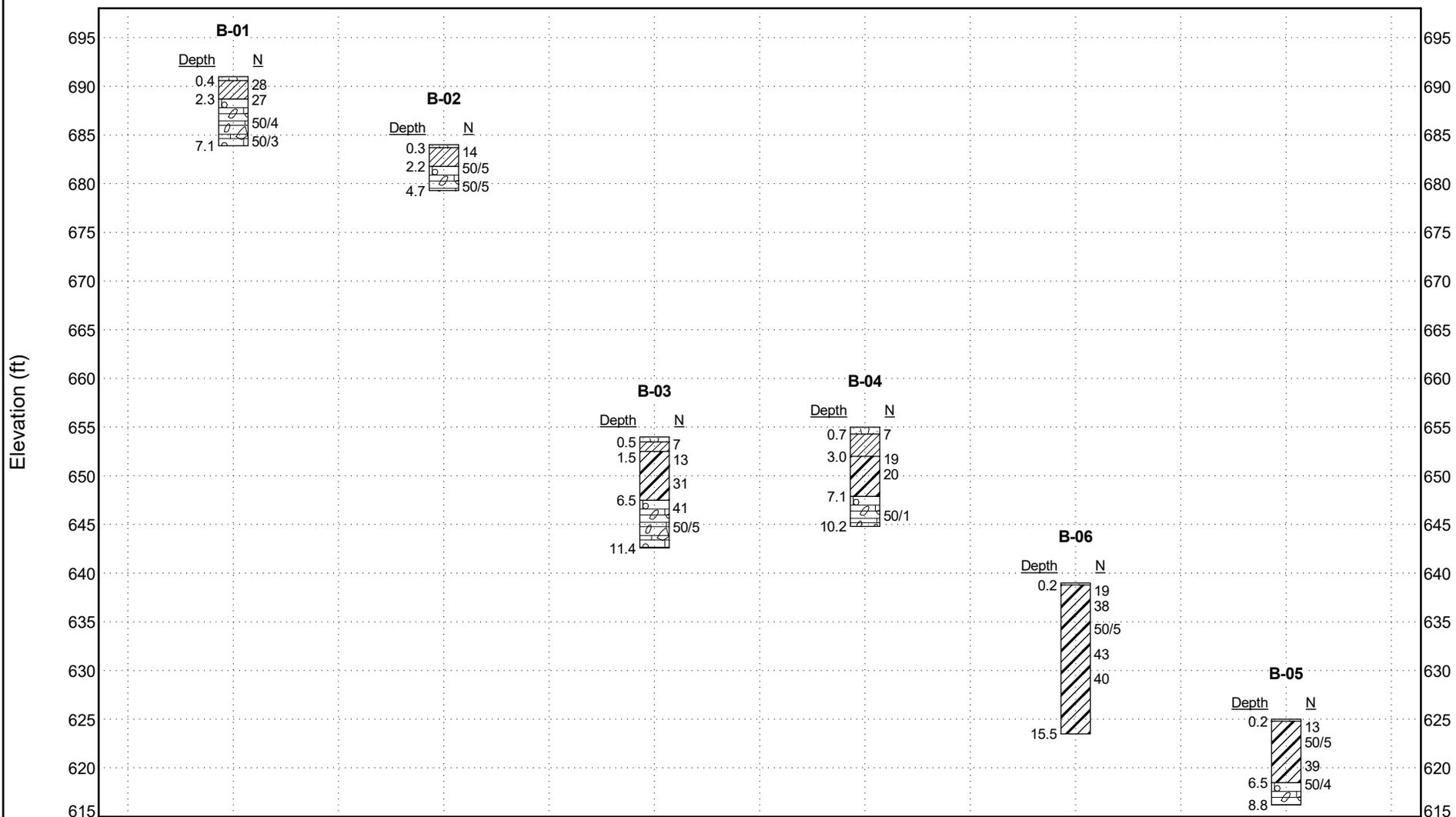
NOTE: The above horizontal boring spacing does not representative the actual distance between borings encountered on-site. Ground surface elevations interpolated to + 1 foot from Digital Elevation Model (DEM) data obtained from the "KYFromAbove" surface elevation and aerial photography database, revised May 5, 2021.
