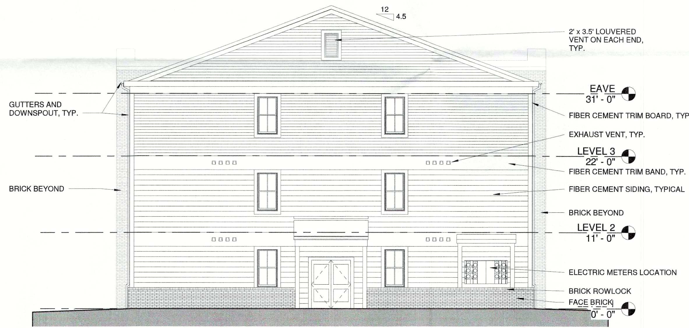
RIGHT ELEVATION BUILDING "A" & "B"
