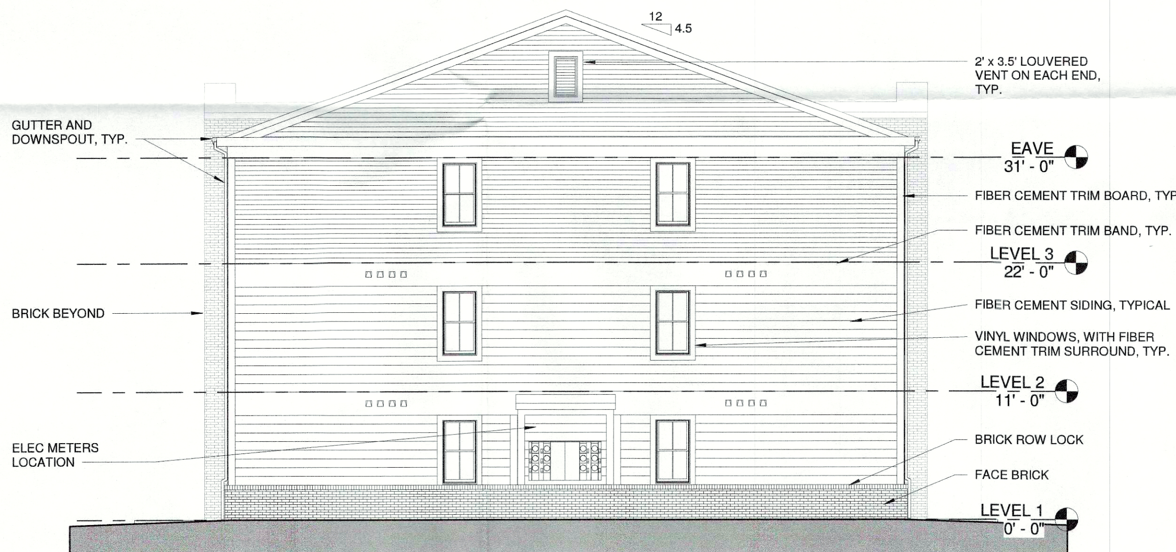
LEFT ELEVATION BUILDING "A" & "B"
