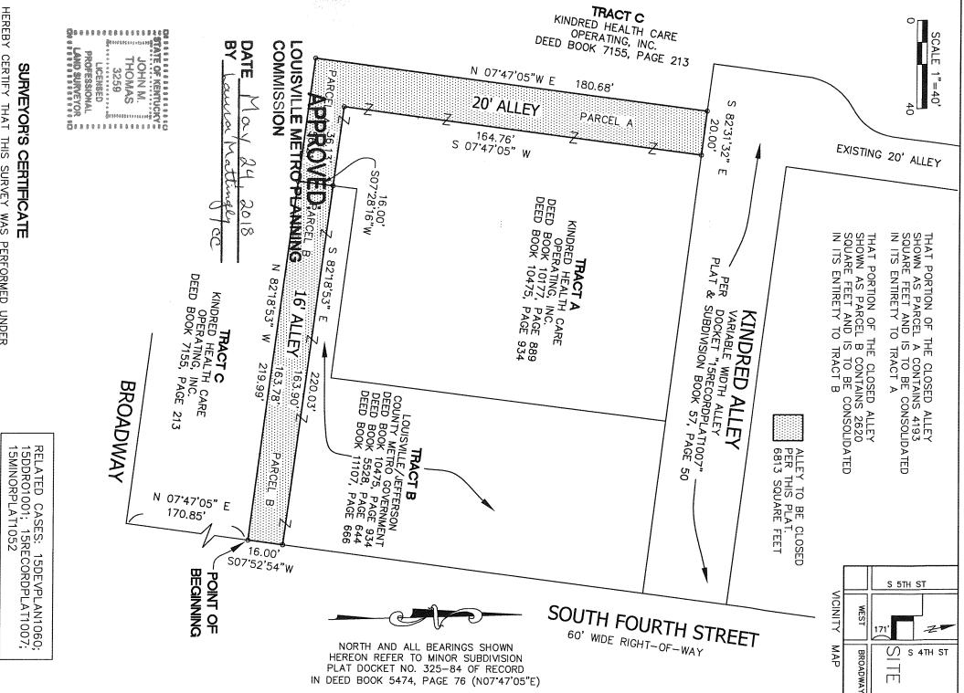
HEREBY CERTIFY THAT THIS SURVEY WAS PERFORMED UNDER MY DIRECT SUPERVISION BY THE METHOD OF RANDOM TRAVERSE WITH SIDESHOTS ON NOVEMBER, 2014. THE UNADJUSTED PRECISION OF THE TRAVERSE WAS 1:20,105. THE BEARINGS, DISTANCES AND TRAVERSE SHOWN HEREON WERE ADJUSTED FOR CLOSURE. THIS SURVEY MEETS OR EXCEEDS THE MINIMUM STANDARDS FOR A URBAN CLASS SURVEY AS ESTABLISHED BY THE COMMONWEALTH OF KENTUCKY, PER 201 KAR 18:150.
