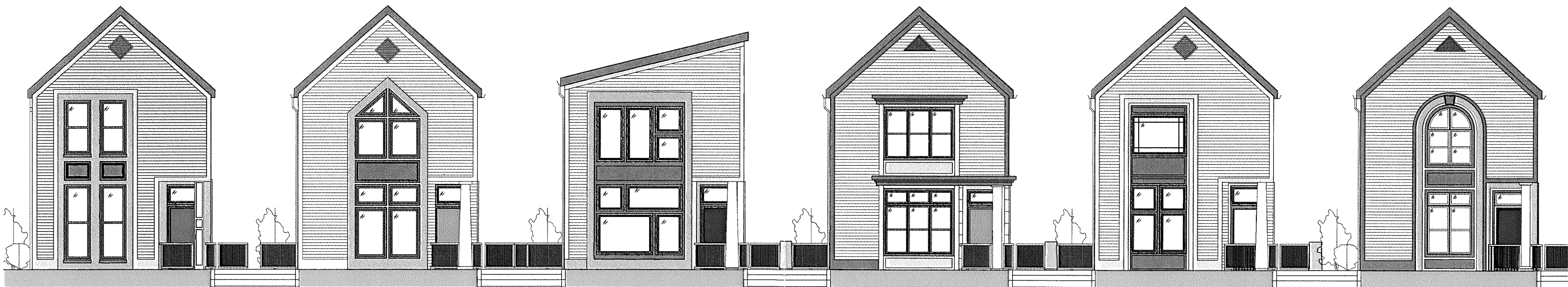
2 ALL UNITS - FRONT ELEVATION OPTIONS A-117 SCALE: 3/32" = 1'-0"
