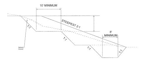
All fill should be placed in lifts not exceeding 8 inches in uncompacted thickness and must be compacted to at least 98 percent of the soils maximum dry density as determined by the Standard Proctor (ASTM D-698). Soil moisture content should be within 2 percent of optimum as determined from the Standard Proctor.
