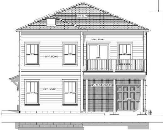
PROPOSED REAR ELEVATION SCALE 1/8"=1'-0"
