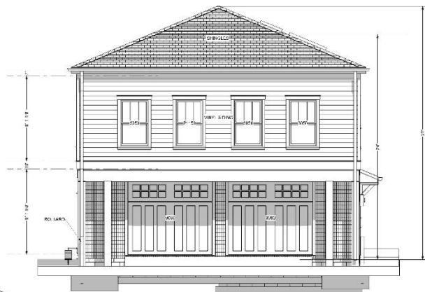
PROPOSED FRONT ELEVATION SCALE 1/8"=1'-0"
