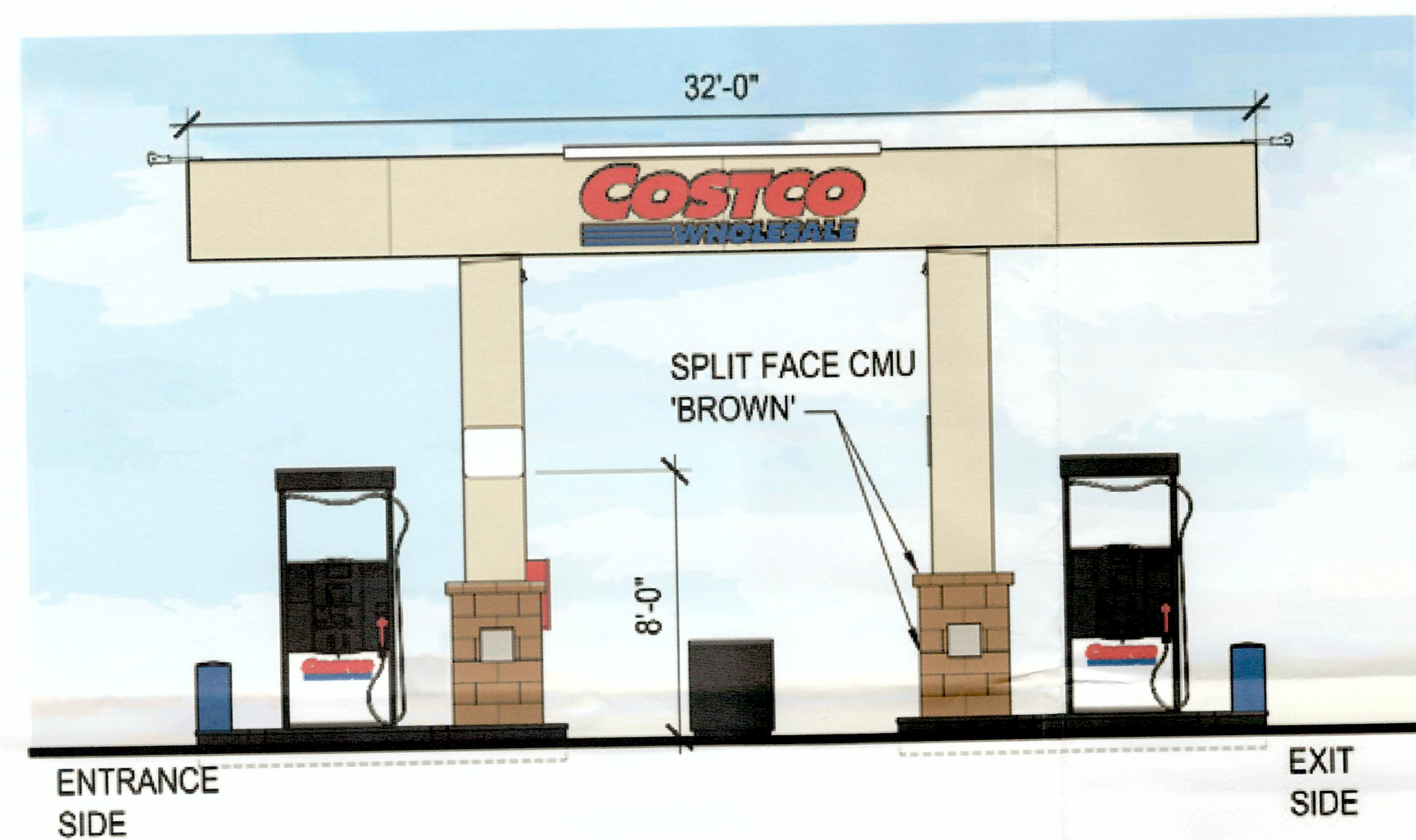
2 NORTH AND SOUTH ELEVATIONS SCALE: NTS
