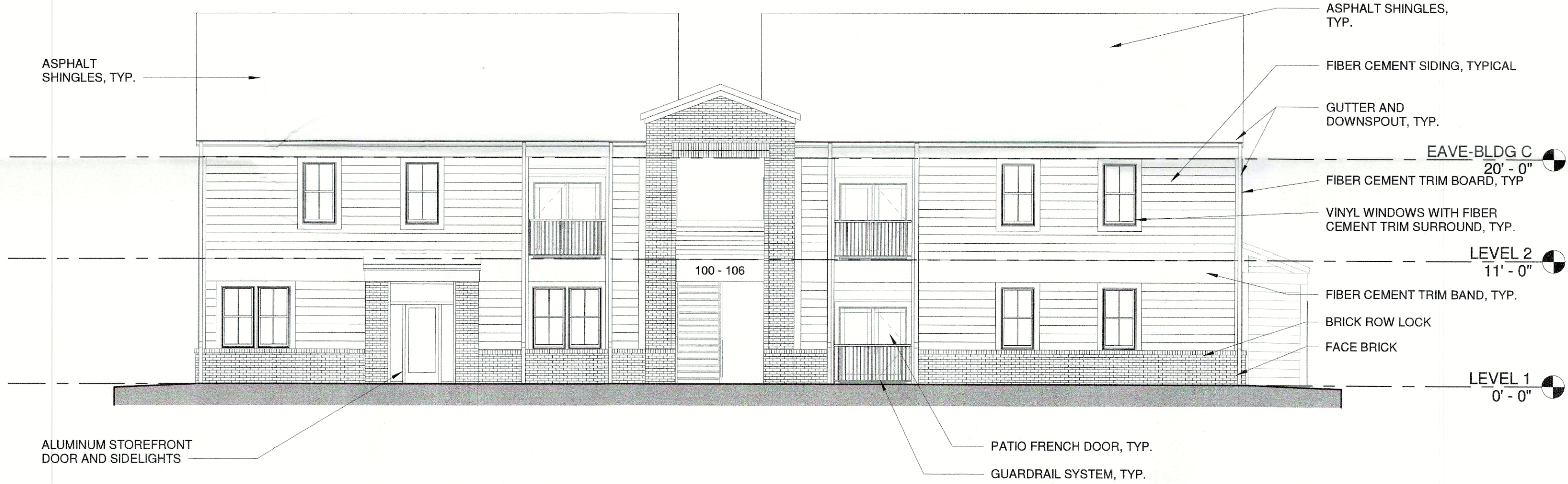
FRONT ELEVATION BUILDING "C"
