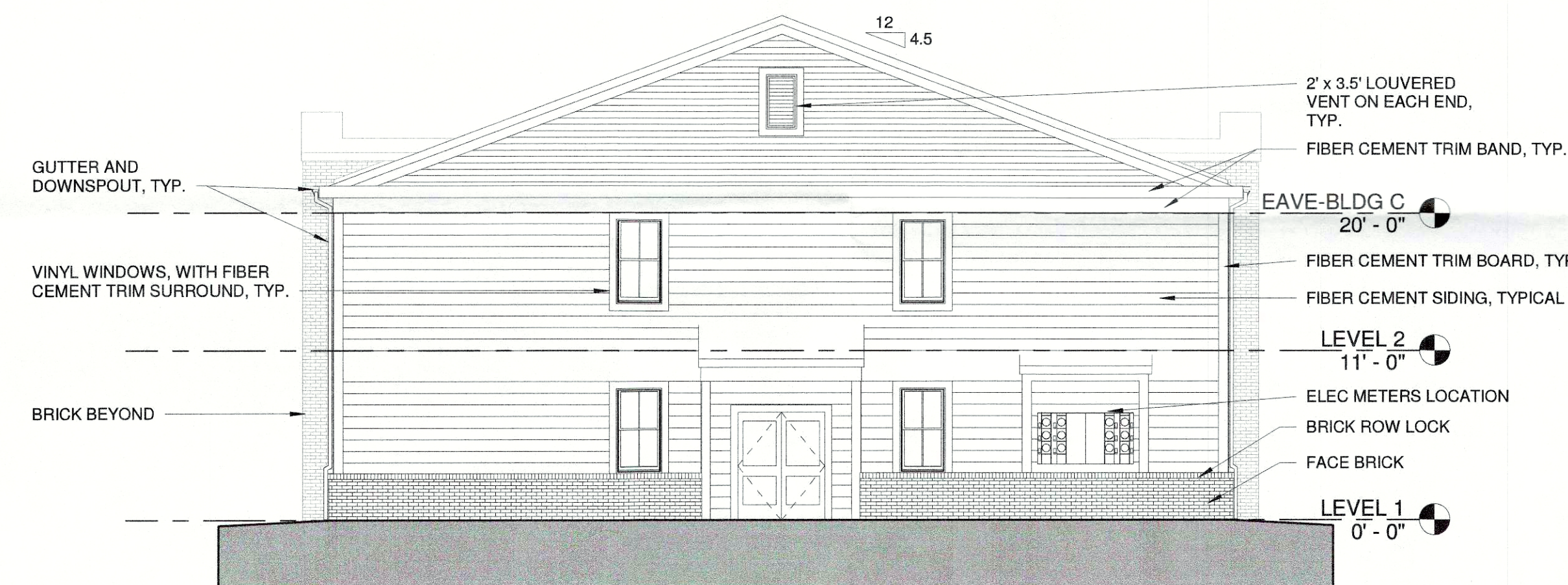
RIGHT ELEVATION BUILDING "C"
