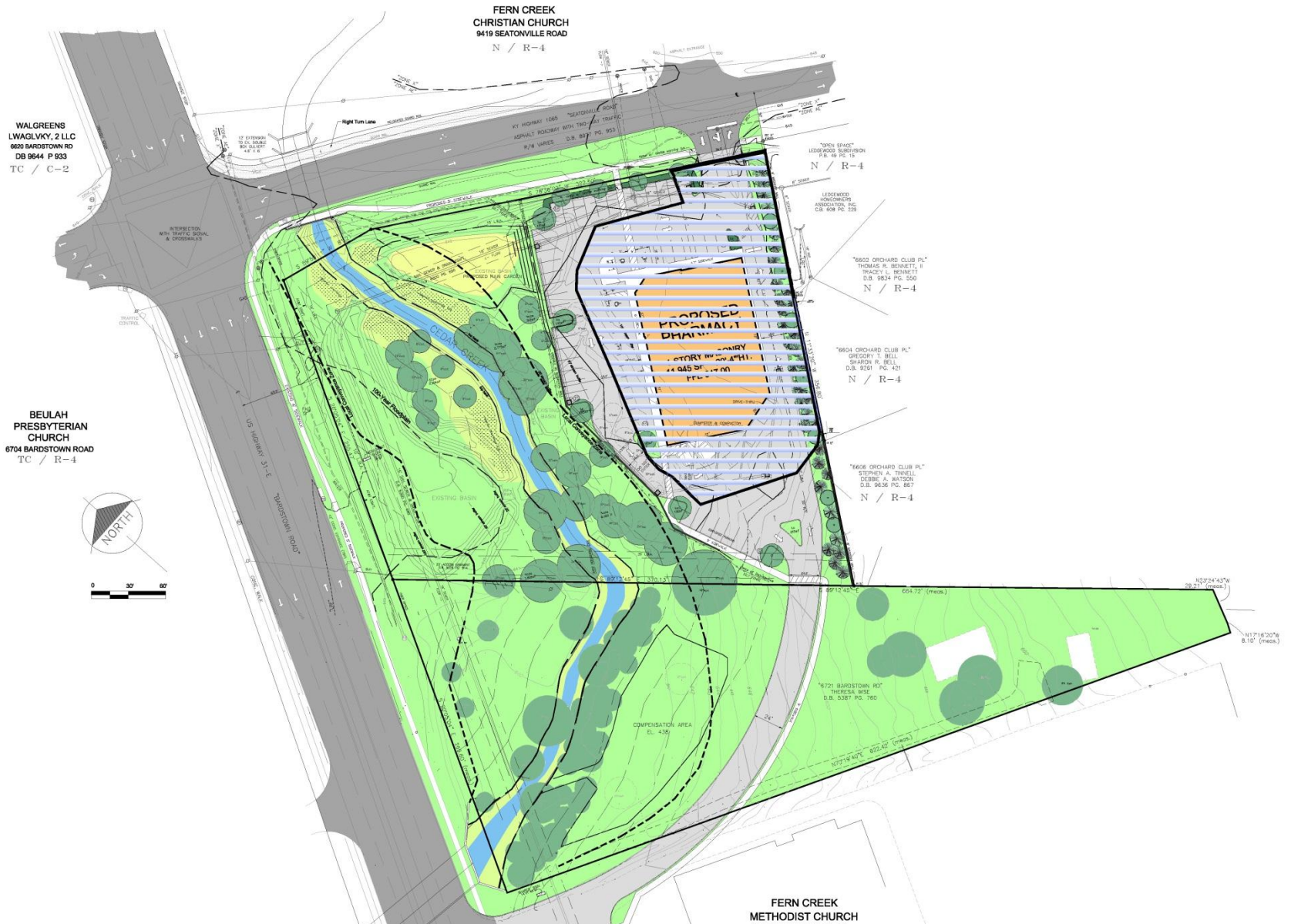
Current proposed CVS plan in darker gray color superimposed on previous approved Branch Bank plan in lighter gray color. Previous proposed Cedar Creek crossing removed, now proposing to utilize existing Fern Creek Methodist Church
