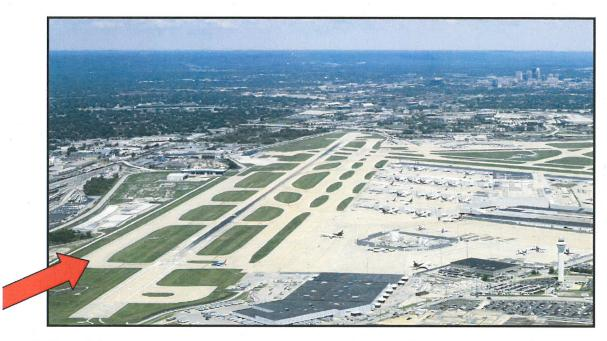
Taxiway Alpha is now 60% complete. In addition to relocating sections of Crittenden Drive, it was necessary to relocate FedEx's aircraft parking area and the company's feeder-truck and employee parking lots to construct the taxiway.
