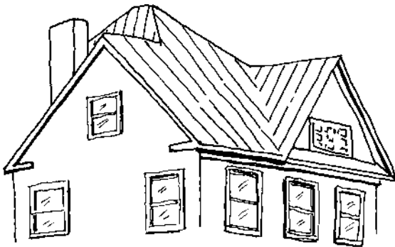
Original metal roofing has a vertical emphasis and a linear quality.
