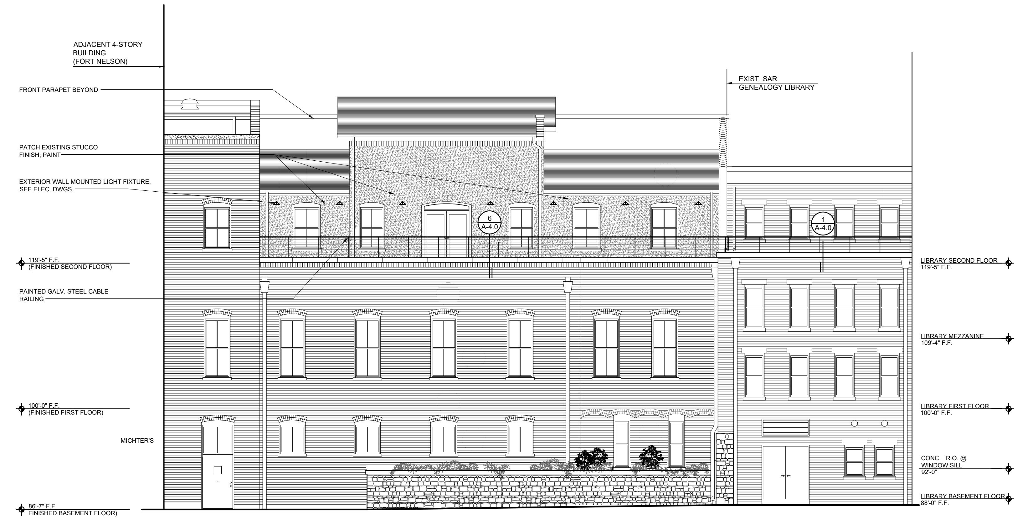
1 WASHINGTON STREET ELEVATION - NORTH 1/8" = 1'-0"
