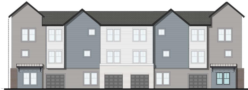
BUILDING TYPE IV - REAR ELEVATION SCALE: 1/8" = 1'-0"
