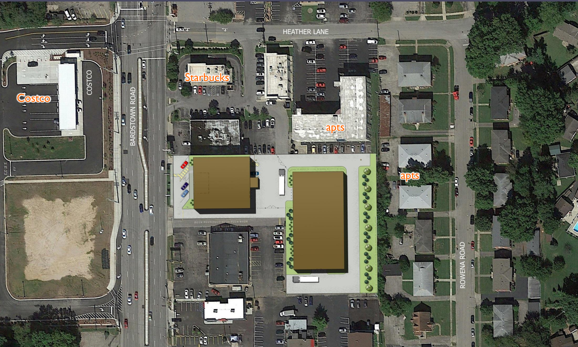
▶ Colored-up site plan with rear (east-side) landscape buffer area; new fence added to help screen site from rear yards of existing apt bldgs.
