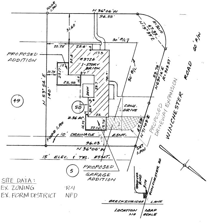
The reference meridian used on this plat to determine the direction of survey bearings has been adjusted to the deed
