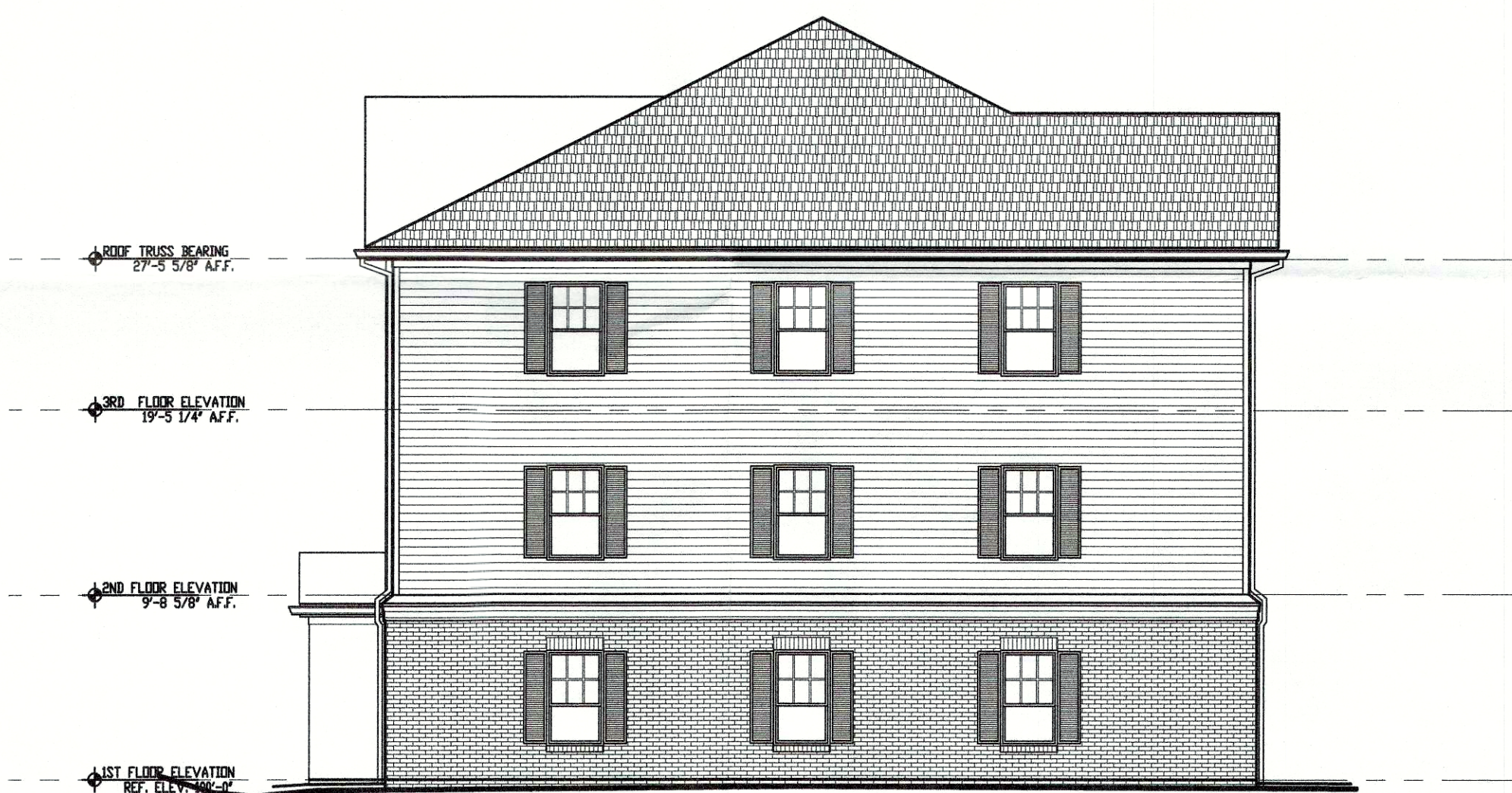
3 SOUTH BUILDING ELEVATION 1/8" = 1'-0"
