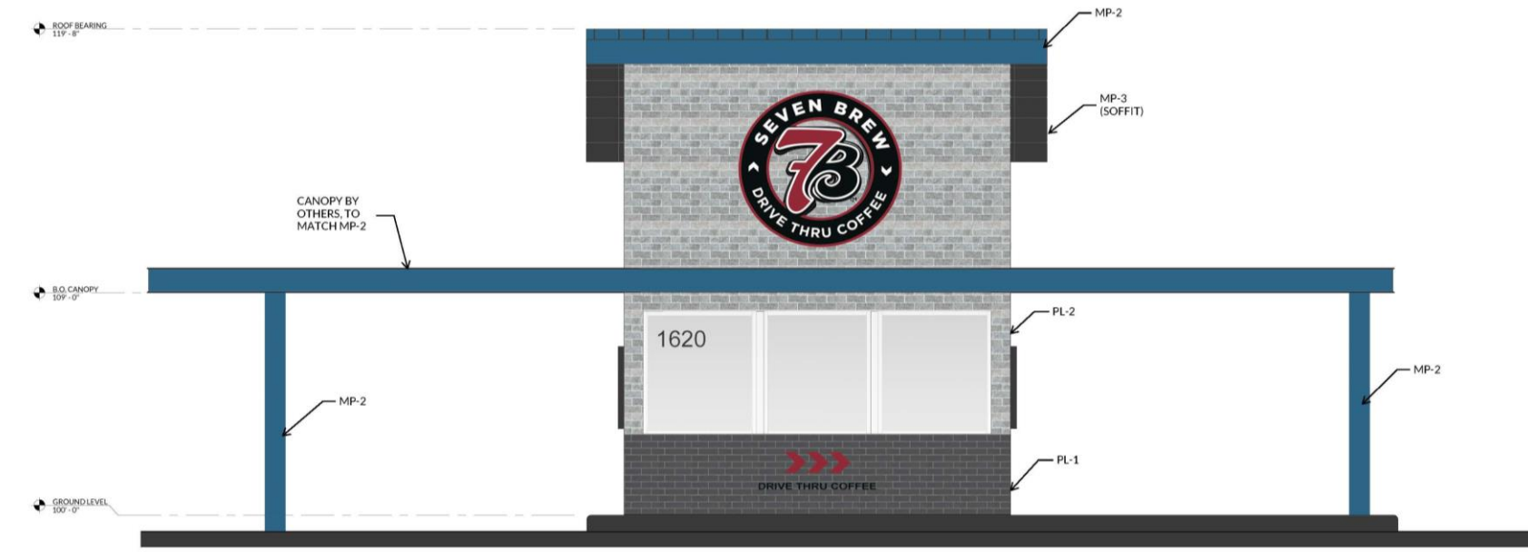
1 EXTERIOR ELEVATION - FRONT 3/8" = 1'-0"
