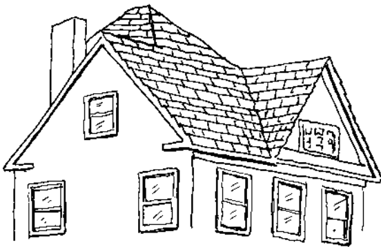
Replacement shingles are uniform and convey no directional emphasis.
