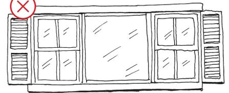
*If replacement of historic shutters is necessary, choose a replacement shutter that appears similar in style, color, size, and material to the historic materials. The replacement shutter should cover one-half of the window were it to be closed.*
