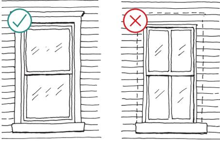
*Do not remove or obscure historic window trim with metal or siding materials. Trim helps visually affix a window within the facade so that it stands out from the wall plane rather than receding into it.*
