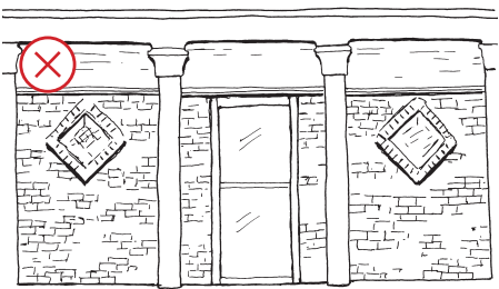
Preserve the original doors and windows on the primary facade. The photo above shows the historic use of expansive plate-glass windows that were used to advertise goods to passersby. The bottom diagram shows how an inappropriate alteration reduces a storefront's transparency, diminishing its historic character.
