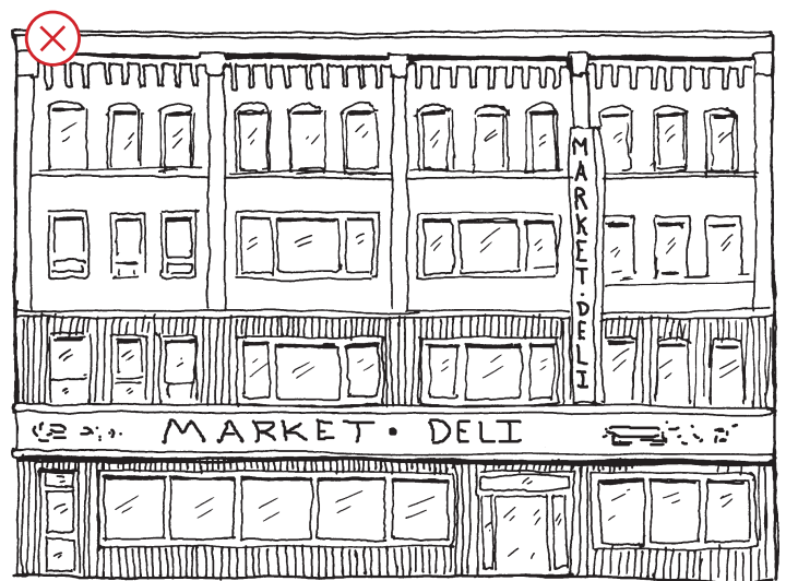
Maintain the original scale, proportion, and organization of architectural elements when repairing a historic storefront. On the left, regular and repeated placement of storefronts, piers, and upper-level windows combine to create streetscape rhythm. On the right, unsympathetic window and storefront alterations disrupt this rhythm and are inappropriate.
