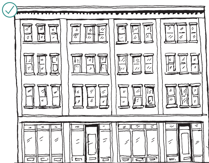
Maintain the original scale, proportion, and organization of architectural elements when repairing a historic storefront. On the left, regular and repeated placement of storefronts, piers, and upper-level windows combine to create streetscape rhythm. On the right, unsympathetic window and storefront alterations disrupt this rhythm and are inappropriate.
