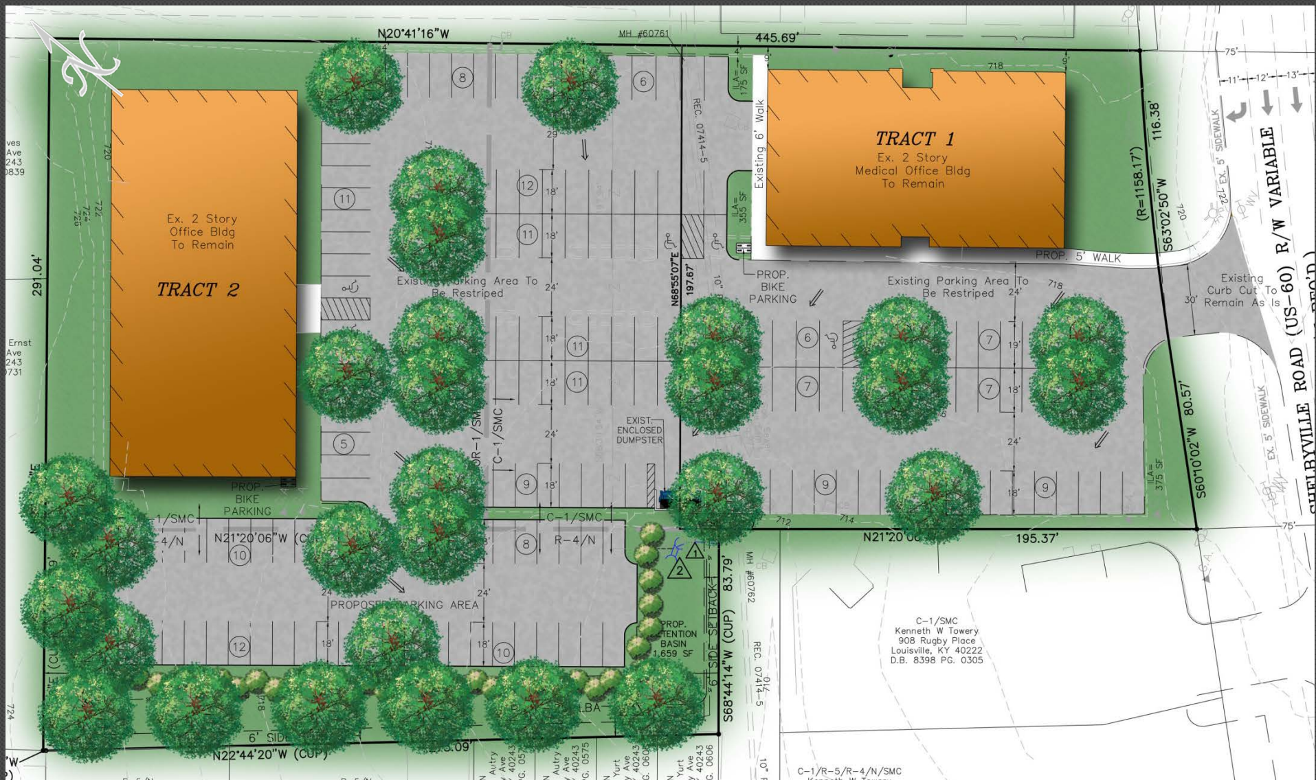
DDD and CUP plans with a variable @ 28 – 34 ft west side yard parking setback, which includes 8 ft high double-sided solid wood fence plus landscaping in buffer setback area.
