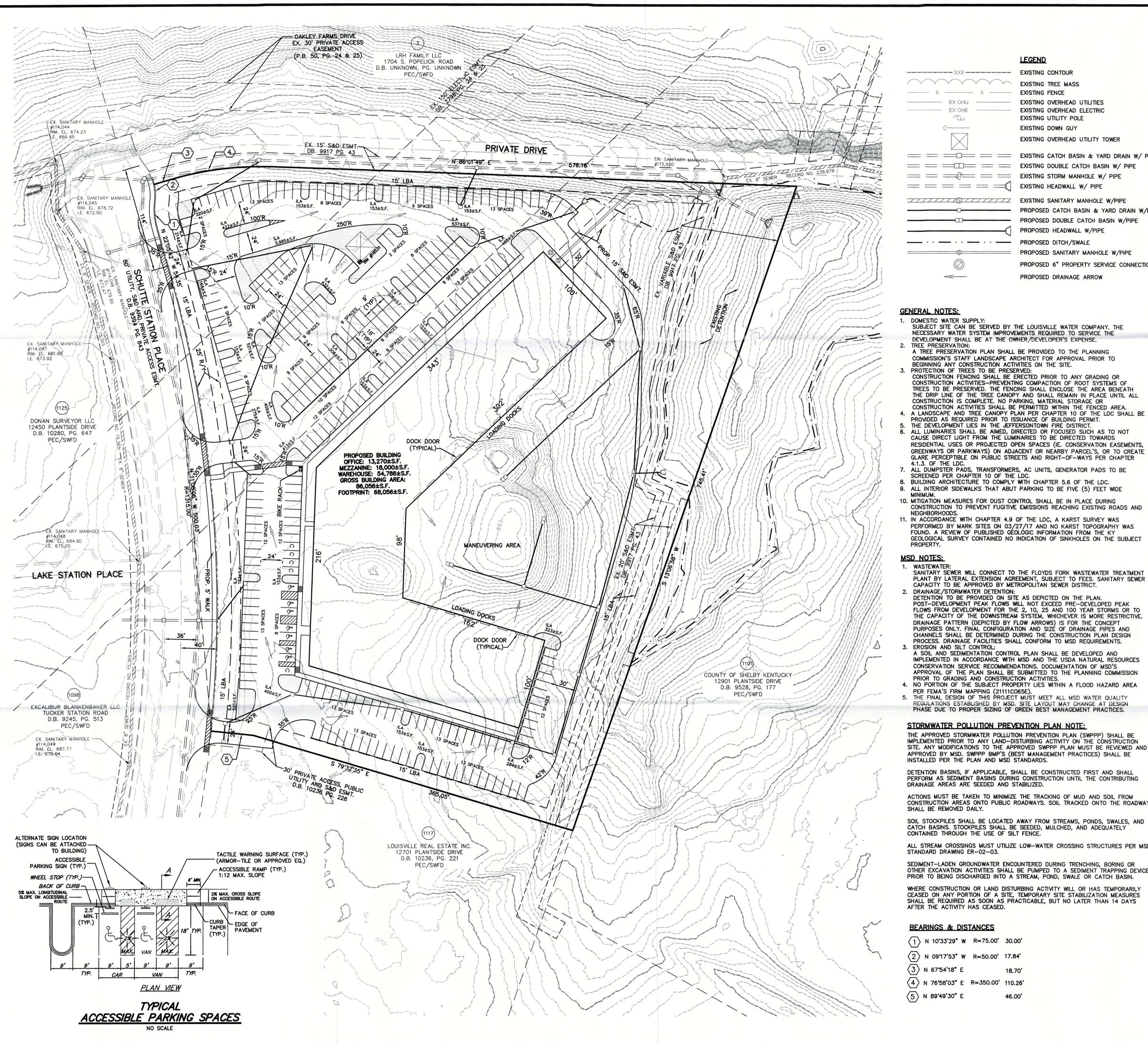
EXISTING CONTOUR EXISTING TREE MASS EXISTING OVERHEAD UTILITIES EXISTING OVERHEAD ELECTRIC EXISTING UTILITY POLE EXISTING DOWN GUY EXISTING OVERHEAD UTILITY TOWER EXISTING CATCH BASIN & YARD DRAIN W/ PIPE EXISTING DOUBLE CATCH BASIN W/ PIPE EXISTING HEADWALL W/ PIPE EXISTING SANITARY MANHOLE W/PIPE PROPOSED CATCH BASIN & YARD DRAIN W/PIPE PROPOSED DOUBLE CATCH BASIN W/PIPE PROPOSED HEADWALL W/PIPE PROPOSED SANITARY MANHOLE W/PIPE
