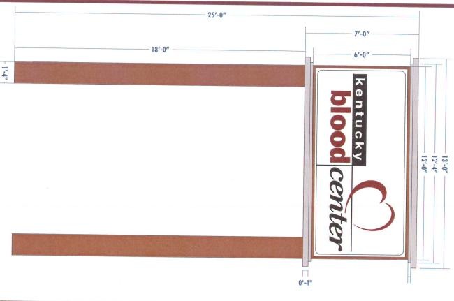
DOUBLE SIDED ILLUMINATED PYLON & CABINET TWO POSTS - DIRECT BURIAL SIZE: 24"d WHITE L.E.D. ILLUMINATION COLOR: SEE CHART ALUMINUM ACCENTS AND POLE COVERS 2" RETAINERS & 1 1/2" H-BAR QUANTITY: ONE (1)
