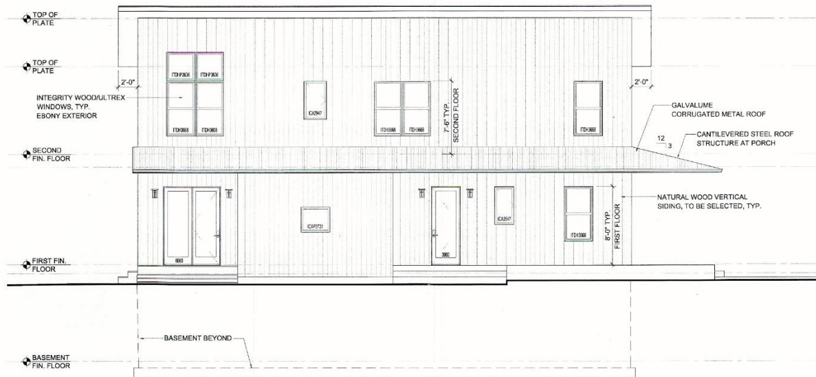
1 PROPOSED NORTH (SIDE) ELEVATION SCALE: 1/4" = 1'-0"
