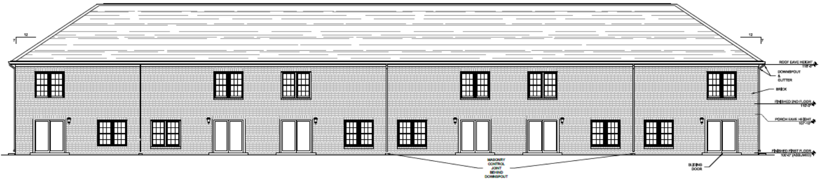
02 REAR ELEVATION SCALE: 3/16" = 1'-0"
