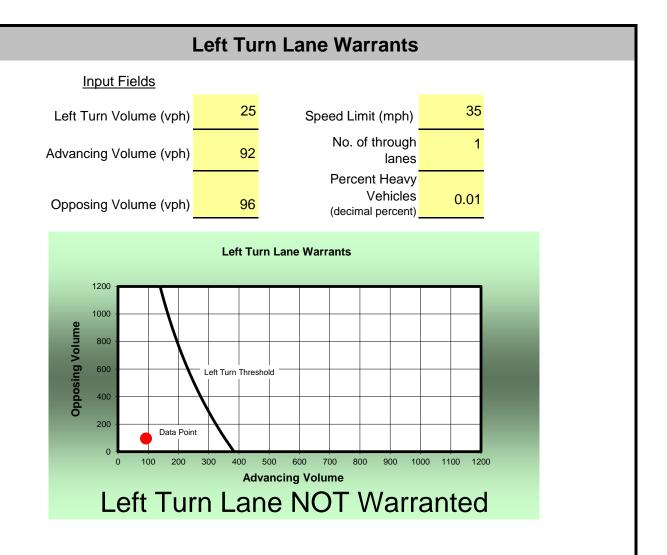
Note: This spreadsheet is intended to supplement the guidance provided in the Auxiliary Turn Lane policy outlined in the KYTC Highway Design Manual. This policy should be fully reviewed and understood prior to using this application.
